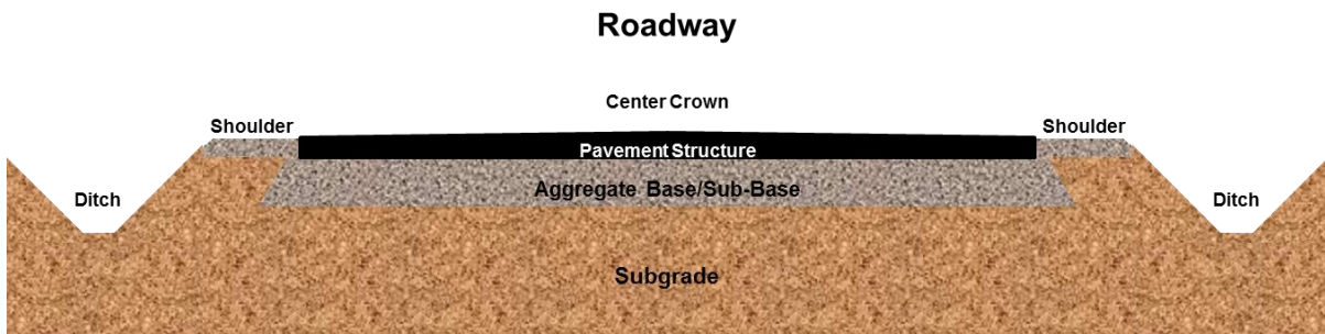
Figure 9 Cross-Section of Parking Lane (Urban Roadway)
